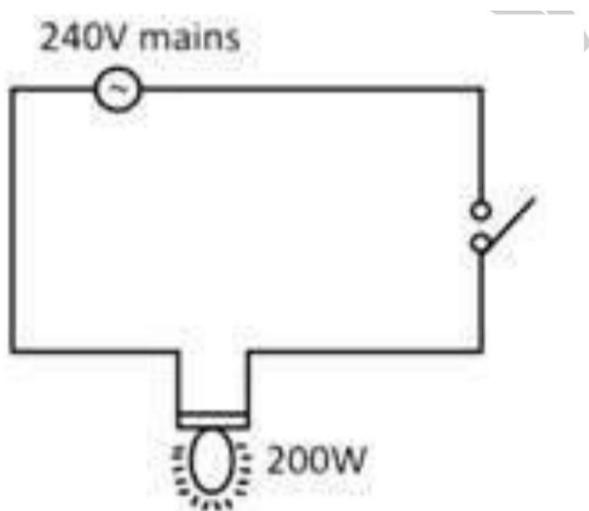
In the diagram above, a 200 W bulb is lighted by a 240 V a.c mains supply. If 1kWh is sold at N40, the cost of keeping the bulb lighted for a day is.
