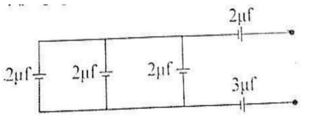
Calculate the effective capacitance of the circuit above
