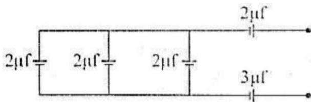
Calculate the effective capacitance of the circuit above.
